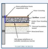
Note: Floating screeds for commercial applications should have a minimum depth of 40mm (BS 8204-7)
